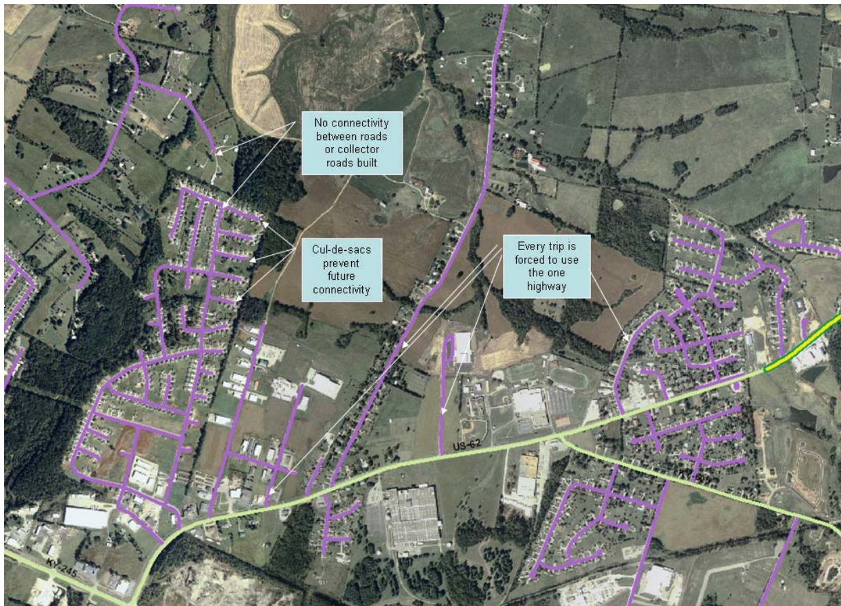
Figure 6: Examples of the lack of roadway interconnection
